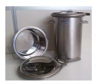
Material St. St. AISI 316 stainless steel, glossy internal finish, external satin finish with completely removed and finished welds. Cover with Silicone gasket and manual closing clamp.
