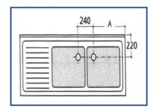
SINK WITH TWO BOWLS + TWO DRIPPING UNITS A = SINK WIDTH /2)-120 mm
